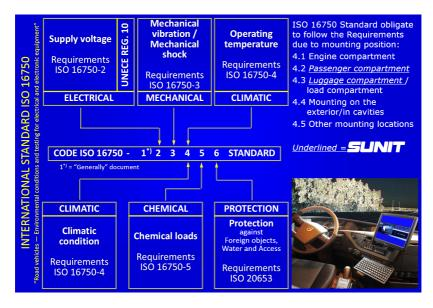
The Vehicle Electronics Standard ISO 16750 determines the Requirements of particular Products and how the Environmentally impacts shall be verified.
