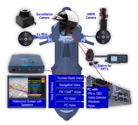
For motorcycles, we offer a comprehensive equipment platform that facilitates work stress. **Sunit Bike-Assist** system is connected to existing Trunked radio enabling voice control between voice-cores to desired priority levels. The Set-up also includes keypads and tripods for special functions as blue lights, quick-resets, quittances, etc.
