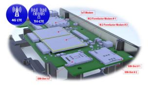
There is optionally platforms for 1 or 2 Modems for Client applications and in addition 1 modem for IoT-interface. Modem-types are selective according to the Clients options. There is Stand-Alone SIM-Slots for all 3 Modems.
