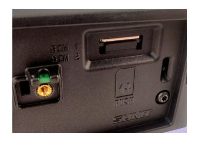
SIM-Cards are easy to install for Client-Modems. They are located at the Front of Computer. The Multi-LTE Applies both LTE-Only
